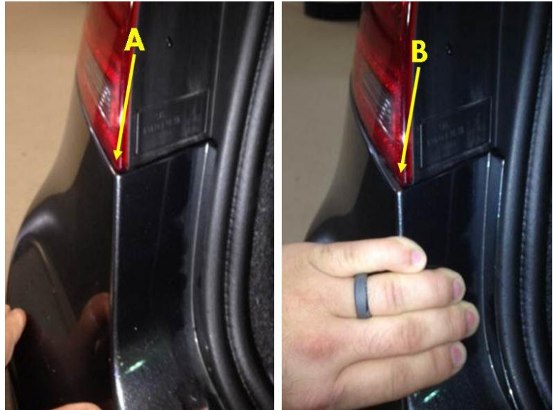
Figure 3. Bumper cover with no free play (A) and bumper cover with free play (B).
