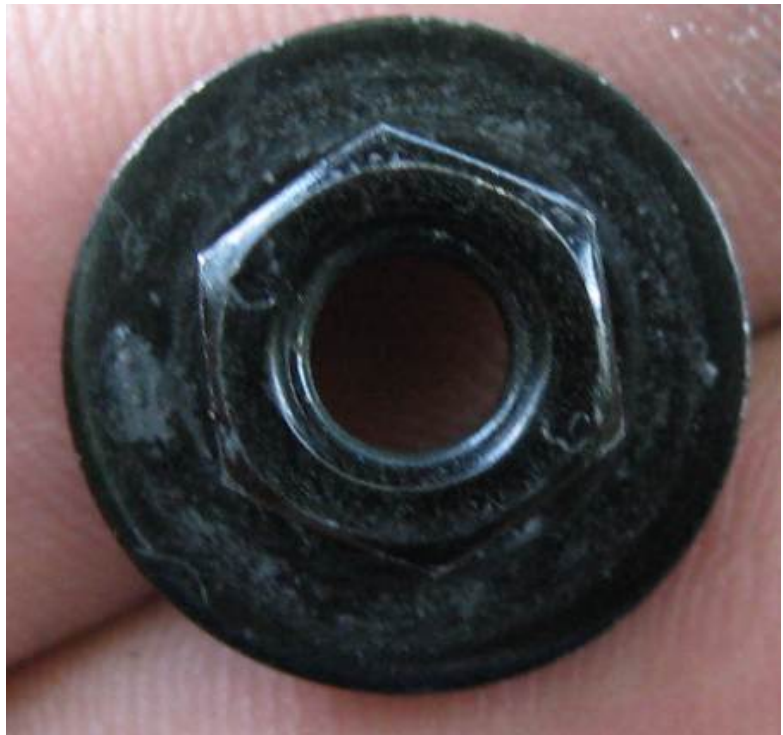
Figure 6. Replacement nuts, part number N 91173301.
