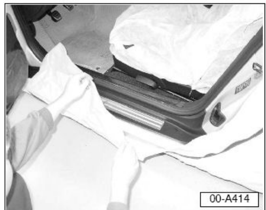
Figure 4. Remove cover from sill.
