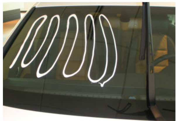
Figure 16. Cleaner applied to windshield.
