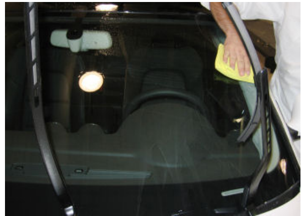
Figure 19. Dry and buff windshield.
