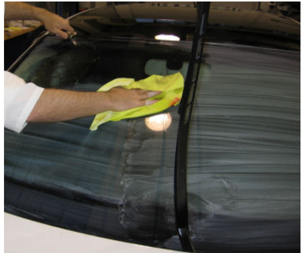
Figure 18. Rinse and wipe windshield.
