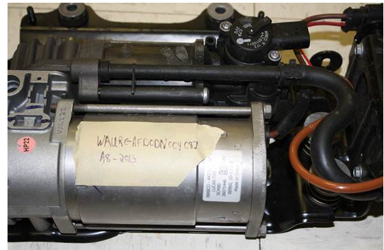
Figure 6. Attach the relay to the compressor and mark both components with the VIN.
