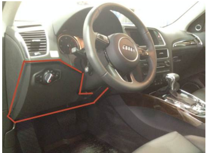
Figure 4. Lower dash cover to be removed.
