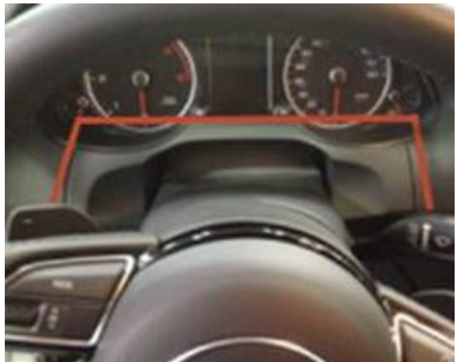
Figure 1. Steering column upper cover to be removed.
