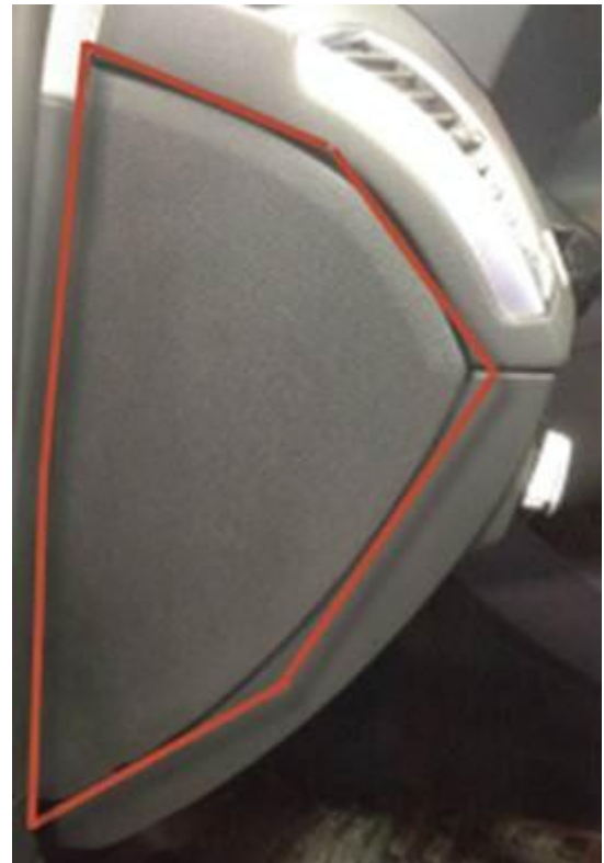
Figure 2. Dash trim side cover to be removed.
