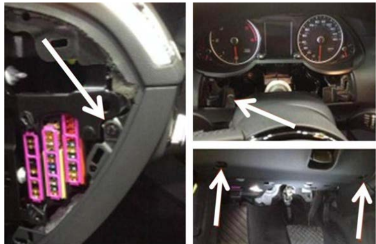
Figure 3. Remove the bolts indicated by the arrows.
