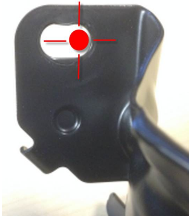
Figure 8. Bolt A should clamp the bracket as shown.
