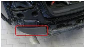
Figure 1. Shield on driver side.
