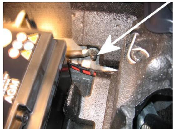
**Figure 1.** Negative battery cable at the body attachment point (white arrow), shown in an Audi Q5.
