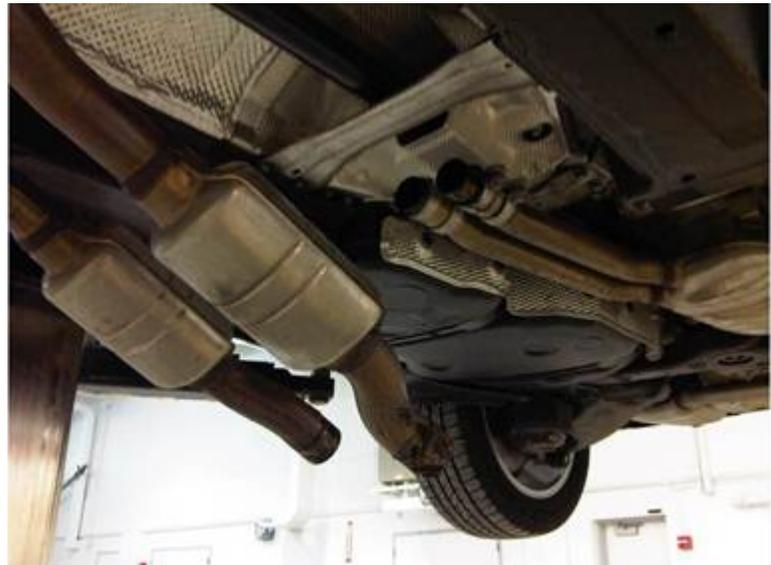
*Figure 7. Lowered catalytic converter pipes*
