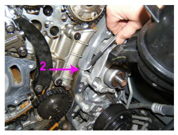
8. Clean out any debris from the T-joint (2) where the right side of the cylinder head meets the engine block.
