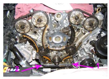
9. Clean out any debris from the T-joint (2) where the left side of the oil pan meets the engine block.
