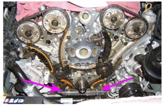
4. Insert a piece of cardboard at the front of the oil pan in the area shown to prevent any contaminants and debris from falling into the oil pan.
