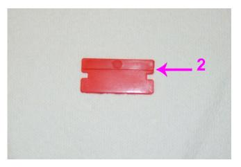
• Use a plastic razor blade (1), that mounts in a scraper device or a hand held plastic razor blade (2), to remove old RTV sealant from a sealing surface.
