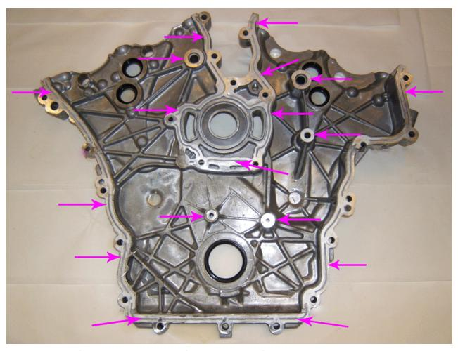
**24.** Apply a 3 mm bead of RTV sealant to the remaining front cover sealing surfaces.
