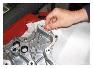
• Position and work the blade back and forth in the grooved areas of the component to loosen and remove the old RTV.
