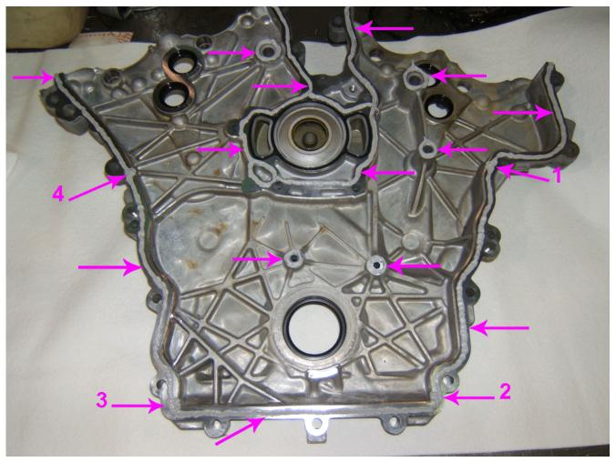
25. This is a typical view of the proper application of the RTV sealant to the front cover, with a 5 mm bead of RTV sealant to the T-joints (1, 2, 3, 4) and a 3 mm bead of RTV sealant to the rest of the sealing surfaces.
