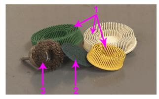
Notice: DO NOT use bristle discs (1), abrasive pads (2), wire wheels (3) or surface conditioning discs to clean the sealing surfaces of engine components.
