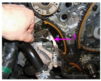
7. Clean out any debris from the T-joint (1) where the left side of the cylinder head meets the engine block.
