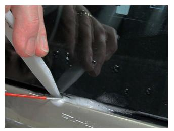
2. Using the spray nozzle attachment, insert the nozzle in the area between the molding and the body and apply a liberal amount of GM Super Lube, P/N 12346241 (in Canada, use 10953474).
