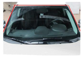
Apply the lubricant along the top and both sides of the windshield opening.
