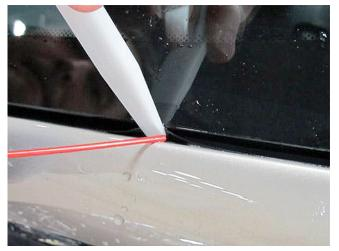
1. Using a plastic trim stick, lift the windshield molding away from the windshield opening exterior surface.
