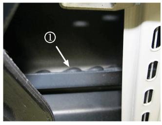
The cause of this condition may be voids in adhesive (1), leaving gaps between the inner door beam and the door skin.
