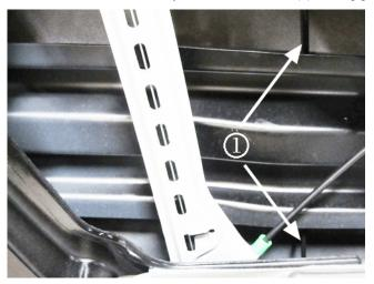
The graphic above shows an example in which a tie strap (1) was passed through a 15-20 cm (6-8 in) length gap where the adhesive was missing towards the center of the door.
