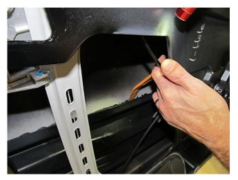
Tip: Use of a trim stick, or equivalent tool, may help to work the sealer into the gap.
