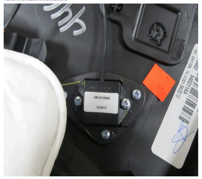
Remove the door panel and verify that the microphone is facing towards the interior of the car as shown in the illustration above. If the microphone is facing the wrong direction, remove and change the direction, reattaching in the proper orientation.
