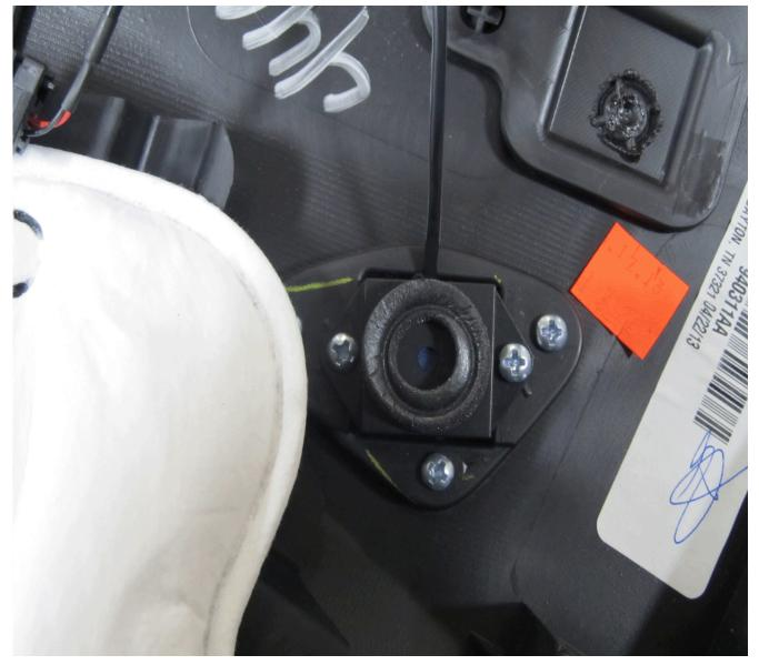
This condition may be caused by the interior noise microphone, located inside each door, facing the incorrect position as shown in the illustration above. In this
