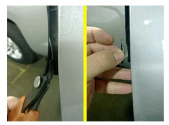
4. Using a pair of snips or sharp scissors, cut along the marked line and discard the removed piece.
