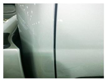
6. Close the door and re-check to make sure the weatherstrip no longer protrudes past the door edge. If it does, repeat this procedure.
