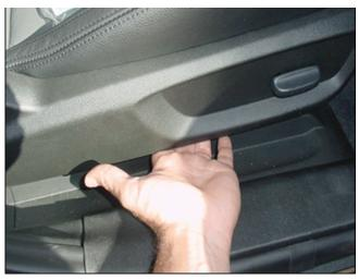
**5.3.** Reaching under the trim panel, pull the metal retaining tab outboard to release the trim panel from the seat frame.
