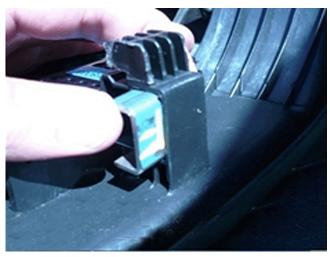
6. Install the two C shaped brackets from the Seat Side Cover Service Repair Kit into the mounting bosses of the new trim panel as shown above.
