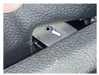
**11.** With the brackets aligned, mark the new screw hole locations through each hook bracket hole onto the plastic seat trim underneath.
