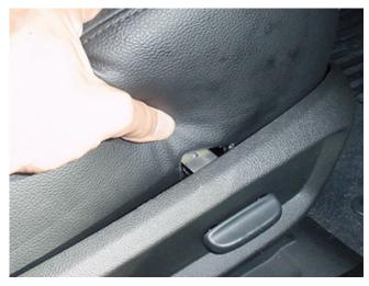
**10.** Push the seat cushion inwards to expose the new brackets that were just installed. Ensure the hook brackets align with the plastic bosses on the trim panel that have the C brackets lodged inside.
