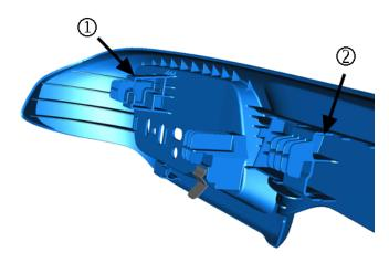
Note: The smaller C bracket goes on the front mounting point (1), the larger one on the rear (2).
