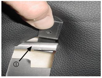
7. Fit the new hook brackets, from the repair kit, to the seat frame by pushing them over the seat frame rail (1) then working them up and down until the angle is right to allow the bracket to clip over the rail.
