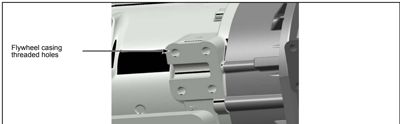
Figure 8 - Flywheel Casing's Threaded Holes
