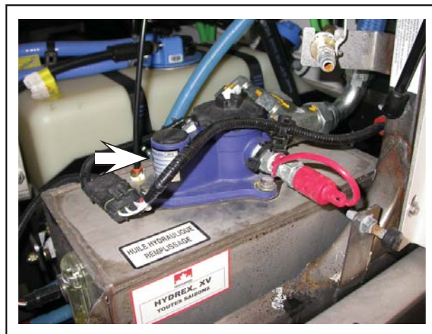
Figure 2 - Filter Housing Location
