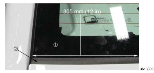
**Note:** Some vehicles may have a urethane sealing issue in the area shown in the photograph. The area of concern is a 305 mm (12 in) section of the rear window glass that begins at the left (driver side) lower corner and ends near the CHMSL. The urethane sealing issue, if present, may allow water to enter the trunk. Look for evidence of a water leak in the trunk.
