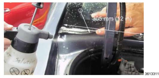
2. Apply a soap and water solution under the water deflector in the 305 mm (12 in) section of the rear glass shown in the photograph.
