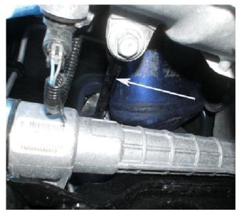
**Note:** Install the new brace on 2006-2007 model year vehicles, GM P/N12617642, using a bolt, GM P/N11570734, to attach the brace to the exhaust manifold/converter. Tighten the bolt to 58 y (43 lb ft).
