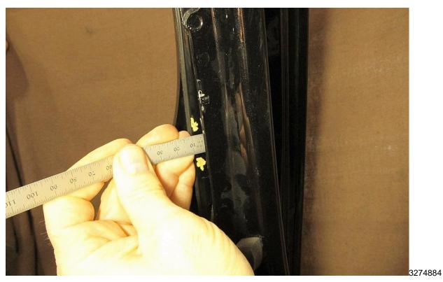
7. Position the spacer to be recessed approximately 2-3 mm (0.078-0.118 in) from the edge of the sheet metal.
