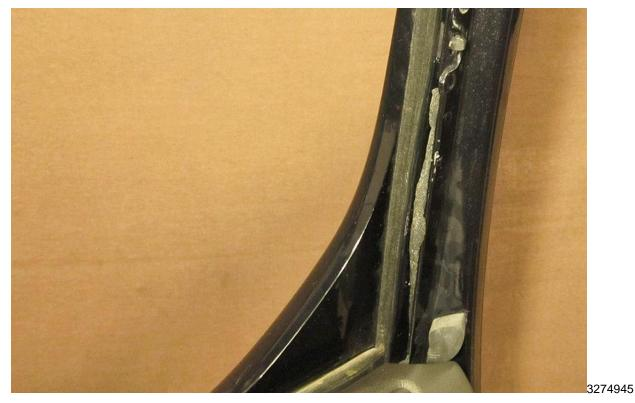
11. Inspect positioning of the weatherstrip to ensure it will not interfere with the fit of the garnish molding.
