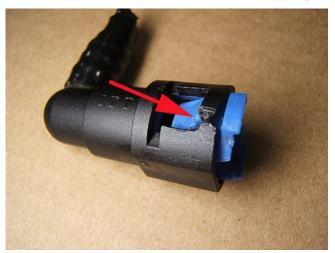
It may be necessary to cut the plastic connector on the hose if the blue plastic retention collar cannot be released. A new connector is part of the new hose assembly.
