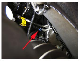
**3.2.** Disconnect the hose from the chassis to canister evaporative emission line.
