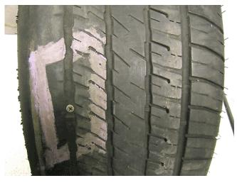
The tire shown above has two non-warrantable conditions. This tire is both badly worn on the inside shoulder (over extended mileage) and has suffered air leakage from a screw still in the tread. Neither of these conditions are warranty related.
