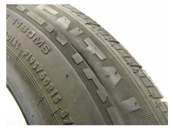
The next sample tire shows both sidewall wear, and cuts in a circum-radial line extending completely around the tire. This damage is the result of extended driving on a tire that is completely flat. The extensive sidewall wear is from contact with the road at that point.
