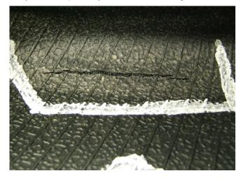
This final example of common road damage is called a "rim-pinch". The air leak is caused by the tire folding and contacting the rim. Frequently this type of damage will cause a sidewall bulge when the tire is inflated, due to internal cord breakage. It is common for this type of damage to only be visible from the inside of the tire. The pictured tire is properly marked and shows a typical tear in the cord. This type of damage is considered road hazard and is NOT warrantable.
