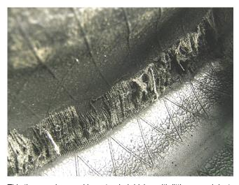
This tire was damaged by extended driving with little or no air just as the tire above it was. This photo shows the inside view. Shredding of the inside may not always be accompanied by obvious exterior damage. In either of these cases, this type of damage is the result of abuse and is NOT a warrantable condition.
