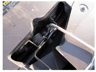
4. With release lever depressed, rotate the release tool to the right (towards driver's side) releasing the hood lock.
