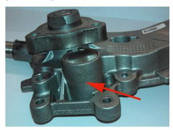
• Slight coolant staining on the underside of the housing.
