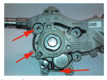
No evidence of coolant leakage on the pump body.
