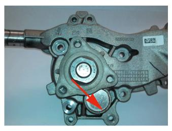
• Slight coolant staining around the perimeter of the cover plate.
