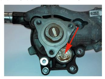
• Significant coolant residue on the cover plate.
