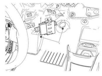
The TCM is located in the vehicle under the left side of the instrument panel (2) as shown in the illustration above.
