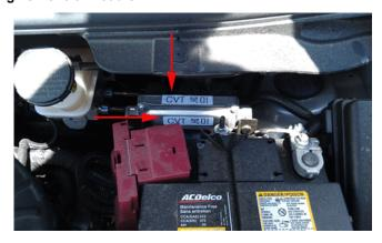
The ECM is located under the hood behind the battery with a label marked CVT as shown in the illustration above.
