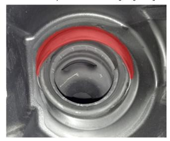
This condition is due to the seal on the fuel tank filler pipe housing not seated properly during vehicle assembly, causing a small EVAP leak and the seal to overlap the fuel tank filler neck as shown in the illustration above.
