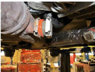
Technicians should follow the procedure below and install two silicone O-rings over each of the exhaust valve springs to dampen the rattle.
