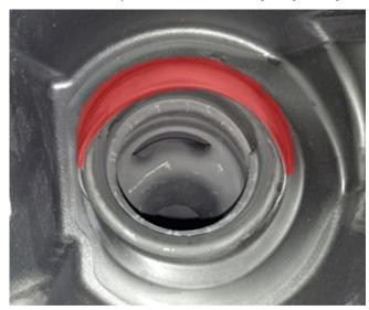
This condition is due to the seal on the fuel tank filler pipe housing not seated properly during vehicle assembly, causing a small EVAP leak and the seal to overlap the fuel tank filler neck as shown in the illustration above.
