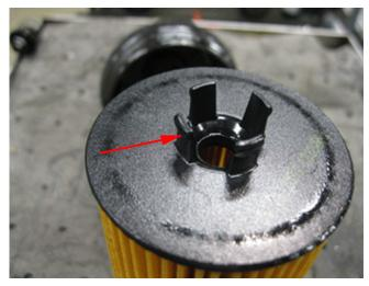
During an oil change, it is possible for the tabs on the oil filter, as shown in the illustration above, to break off and fall into the oil filter housing.
