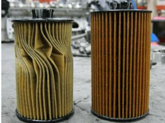
Shown in the illustrations above is an oil filter that was installed improperly, which caused the oil filter to be smashed and cannot close the oil filter drain check valve.
