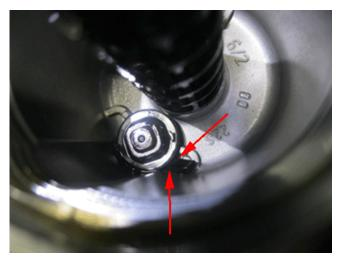
This piece may become lodged under the oil filter housing drain check valve, causing it to remain open when the new filter is installed as shown in the illustration above. This will allow oil to drain back into the oil pan and reduce the pressure allowed to the engine.
