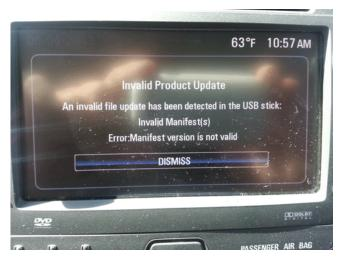
Note: If the following screen above is shown on the screen, the radio already has the latest calibration installed and no further action is required.
