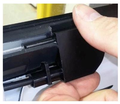
If the cable pulley cover completely disengages, the pulley can come off and cause the cable to bind, see photo below.
