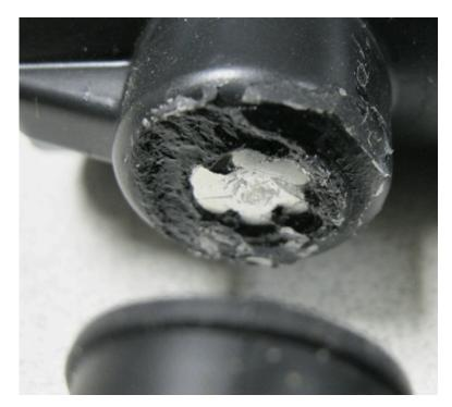
This type of damage is caused by prying up on one end of the coil assembly. The EN-6009 tools must be used to lift up at equal angles at both ends of the coil assembly.
