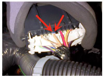
Inspect connector X109 before disconnection. Terminal A5, motor circuit (1552) is visibly backed out in the image above.
