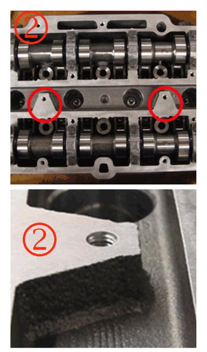
If the cylinder head is first design, then replace the cylinder head using the latest part number in the catalog.
