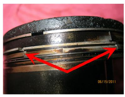
If cracked piston ring lands are found, then inspect the cylinder head to determine first or second design. See photos below: First design (call out #1)
