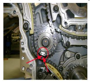
The left camshafts will be aligned as shown when in Stage two timing position.
