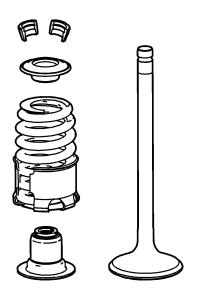
If single bank misfires are found, then remove the valve cover of the affected bank and check the valve springs for missing harmonic stabilizers (see picture below.) Replace the valve spring assemblies if the stabilizers are not present and retest for the misfires.
