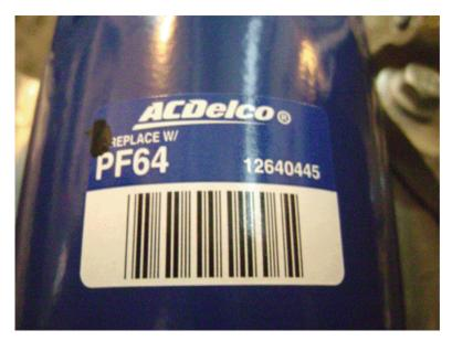
Caution: The PF63 will fit the engine. However, it is significantly longer and it is possible it could be damaged if the suspension goes to full compression.
