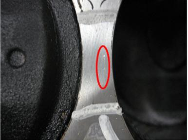
Small surface pock marks or pitting appearance on the deck surface is normal and engines should not be replaced for such appearance as they do not connect to coolant passages and cause a leak path that generate engine misfires.
