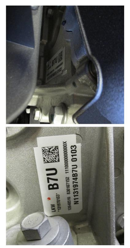
Example: Engine Unit Identification number found on the timing cover: N1131974B7U 0103
