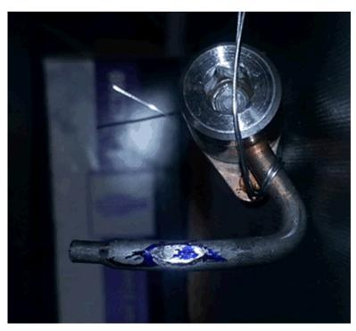
If contact is noted the dealer needs to call PQC for a replacement engine. (PER PIP5114) Pictures of normal crankshaft marking that are not caused by the oil squirter making contact:
