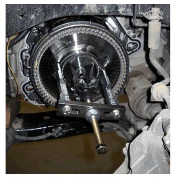
**Important:** To install bearing use Special Tools DT-22928-B Seal Installer per SI, as damage may occur if the proper tools are not utilized. Proper bearing orientation is the writing up or visible to technician.
