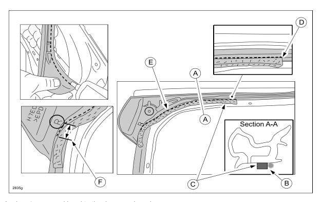
7. Apply a 4 mm round bead to the door panel as shown:
