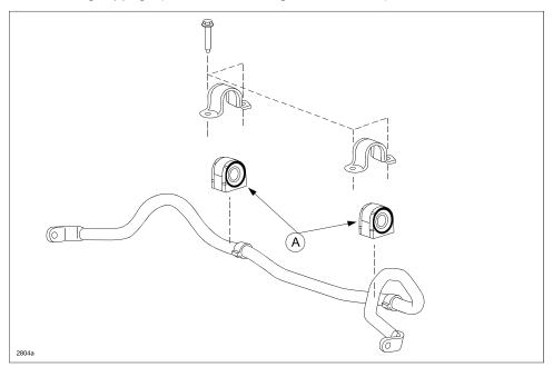
NOTE: To prevent noise from occurring, never apply any type of grease or lubrication to the front or rear stabilizer bushings.
