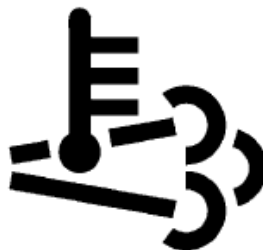
High Exhaust System Temperature (HEST)
