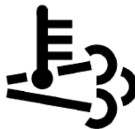
High Exhaust System Temperature (HEST)
