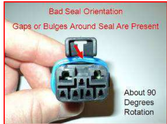
Fig. 4b: Improper Orientation
