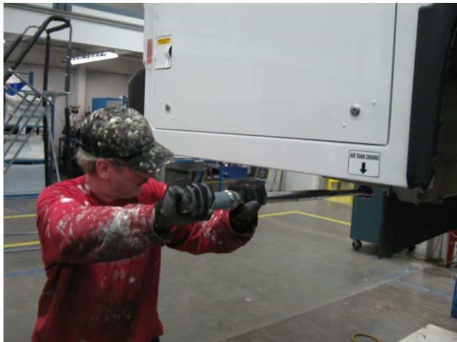
Figure 6: Torque Bolts to Specification
