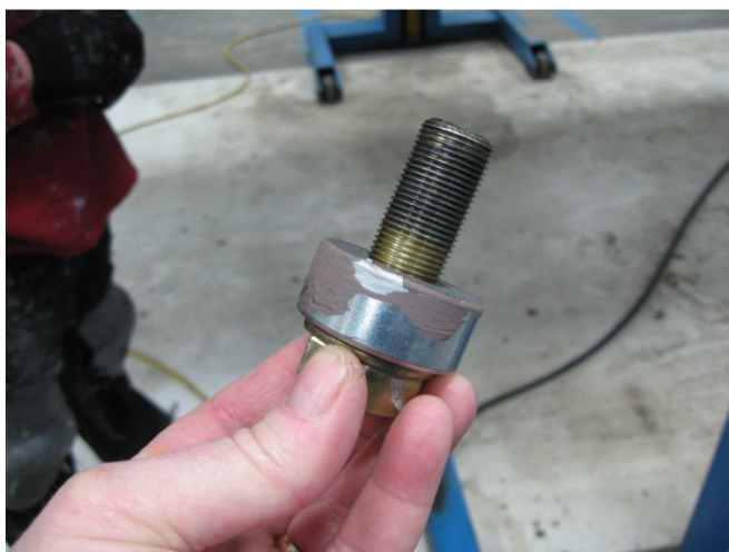
Figure 2: Removed Bolt, Washer and Spacer
