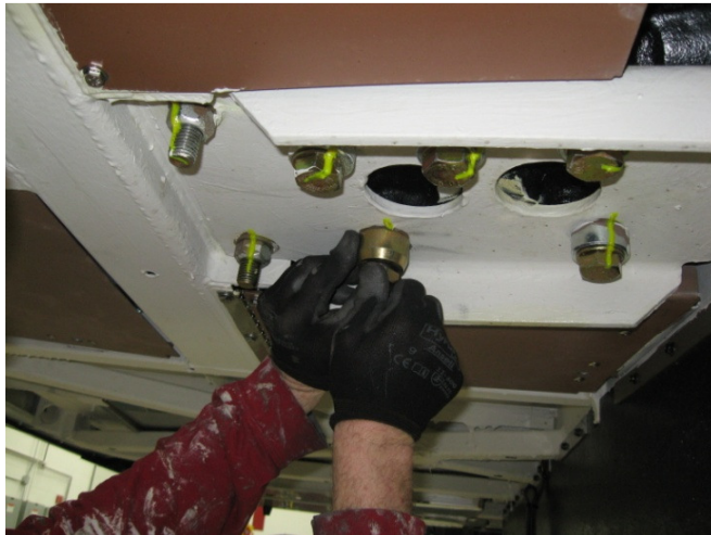
Figure 5: Hand tight bolts
