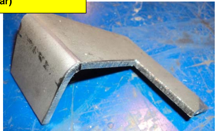
Gusset Shown for Street Side radius rod bracket (curb side is similar)
