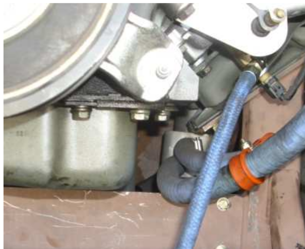
Figure 22: Lateral Engine Brace
