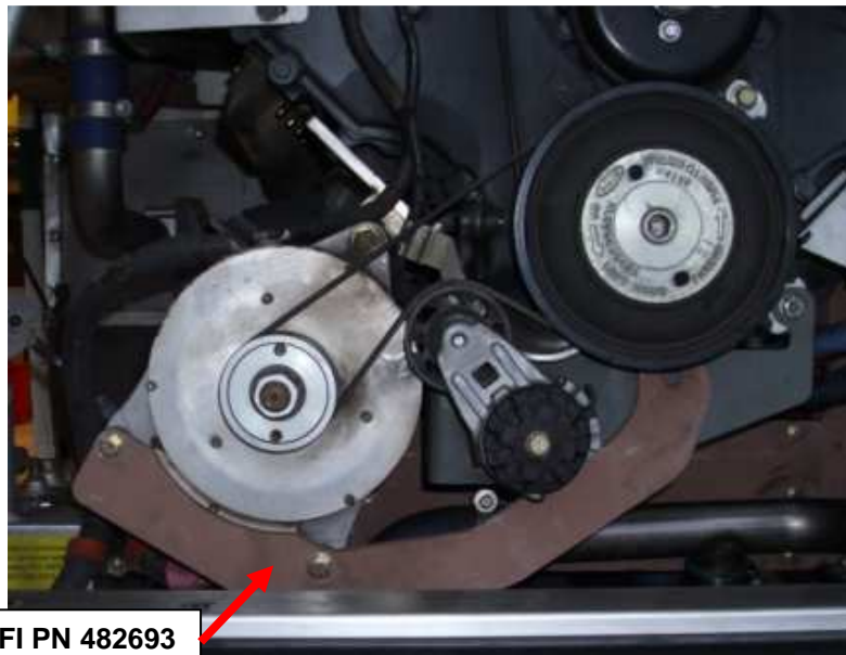
Figure 30: New Alternator Bracket
