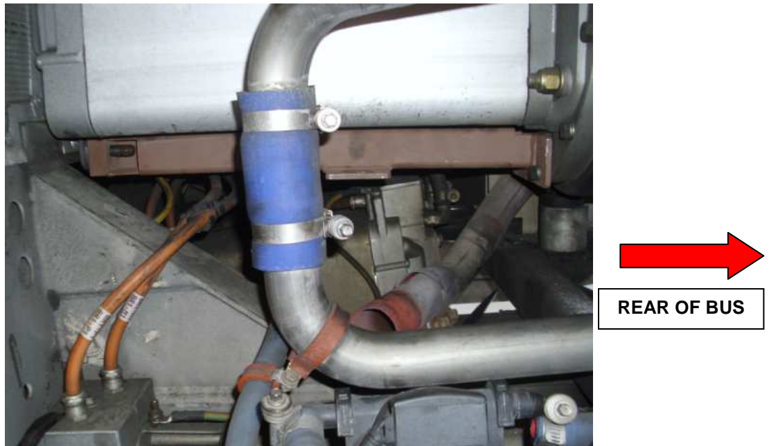
Figure 26: Assembled generator support assembly
