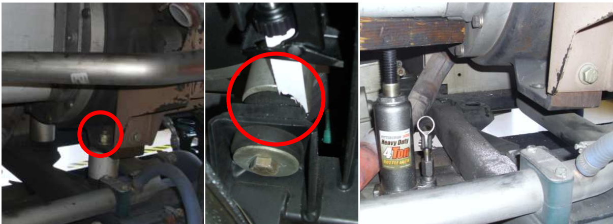
Figure 15: Bell Housing Spacer Removal
