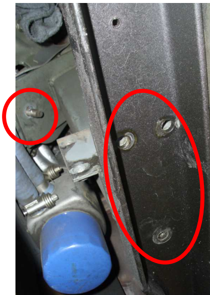
Figure 17: CS Mount Removal
