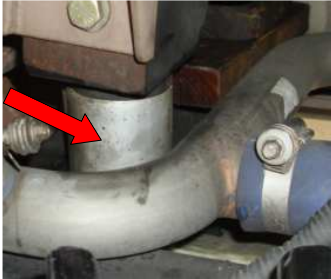
Figure 25: Temporary Stand for Engine and Cradle
