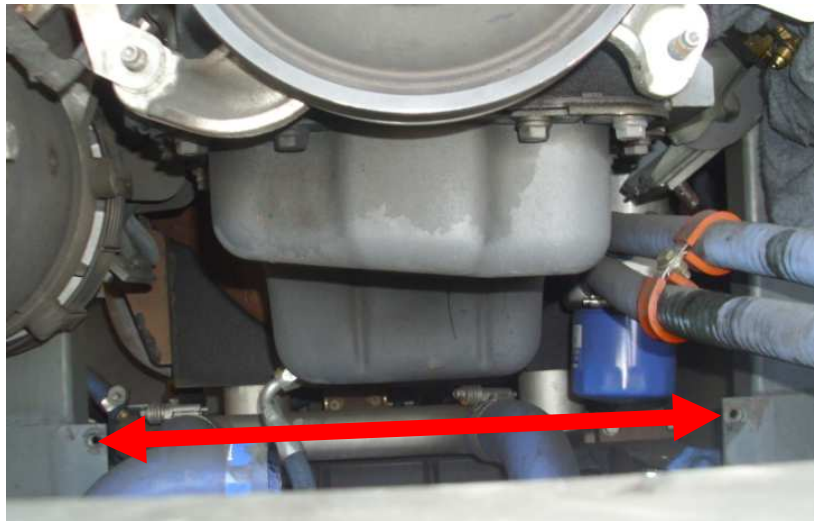
Figure 13: Front Engine Center Brace
