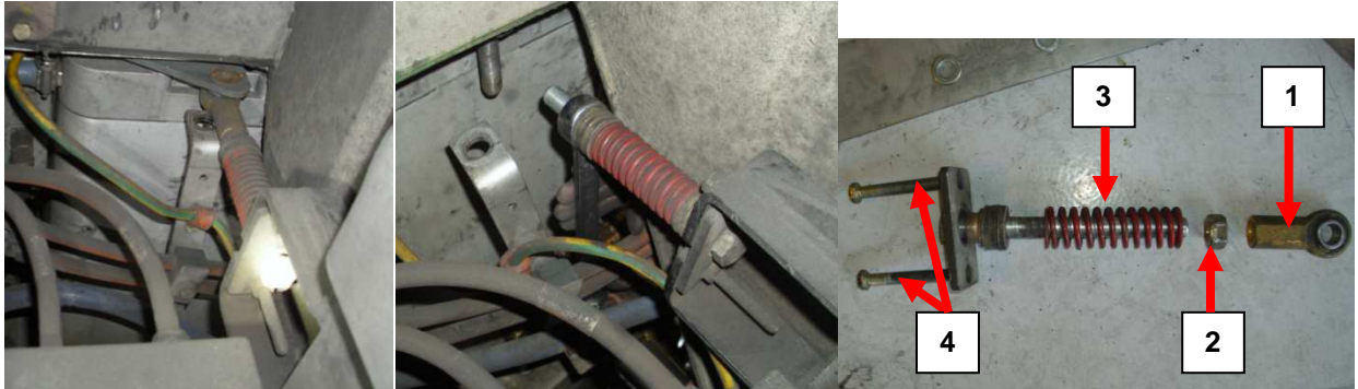
Figure 12: Generator Mount Assembly
