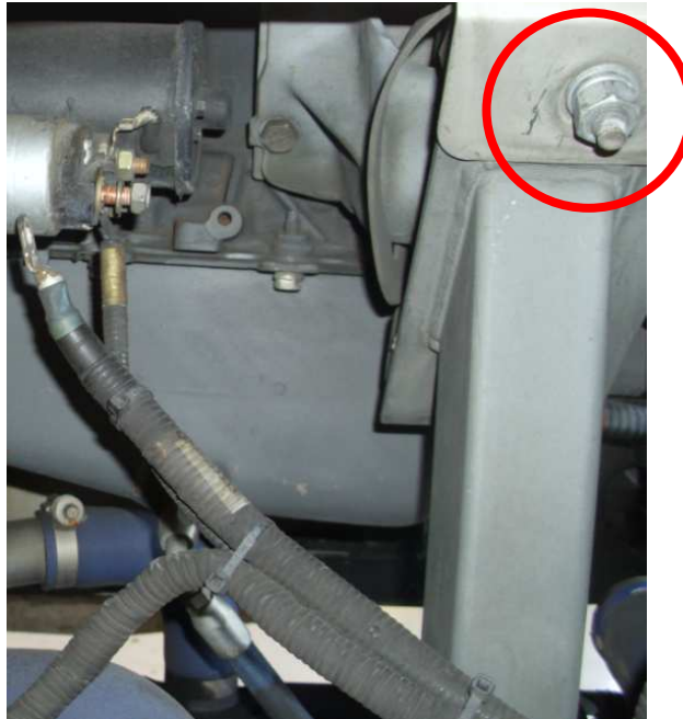
Figure 14: Front Engine Center Brace
