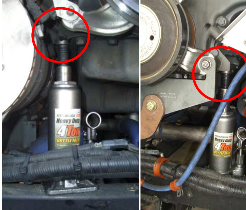
Figure 16: Bell Housing Spacer Removal/Engine Tabs
