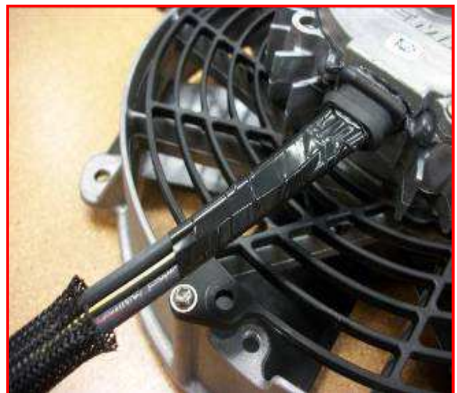
Figure 10: Fan Harness Taped
