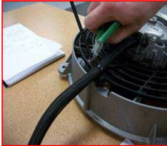
Figure 15: Securing and Trim of Zip Tie
