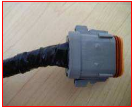
Figure 36: Wires taped on J1939 Connector
