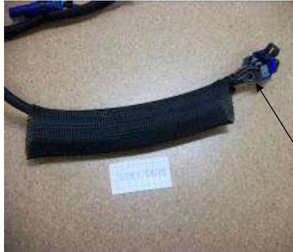
Figure 18: Braided Material Over Main Harness
