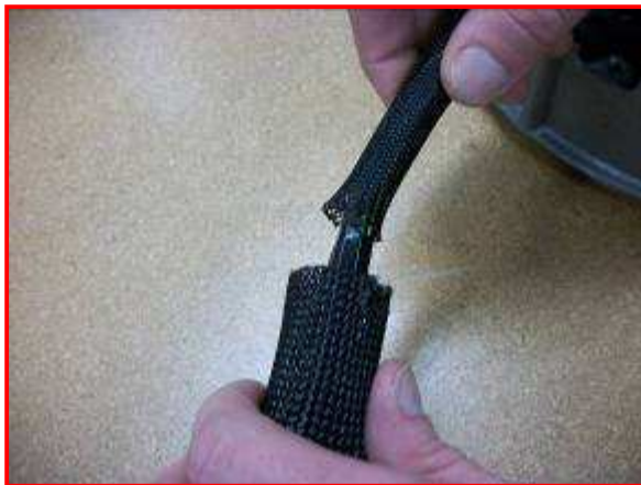
Figure 29: Braided Sleeve Before Extension
