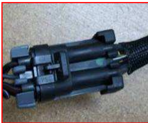
Figure 23: No Seal Visible, Correct
