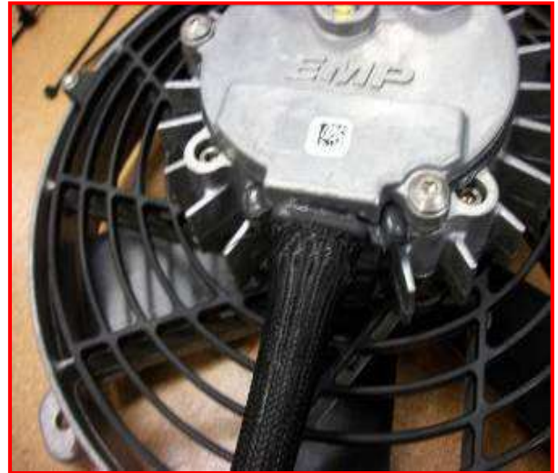
Figure 12: Sleeve Over Header
