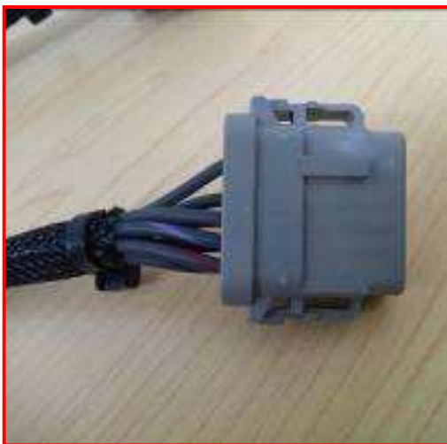
Figure 34: Wires exposed on TMC Connector
