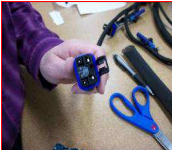
Figure 19: Di Electric Grease on Connector
