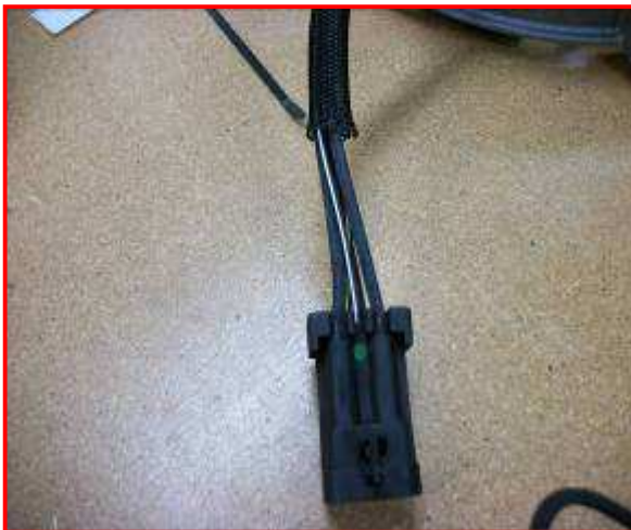
Figure 16: Exposed Wires on Fan Harness
