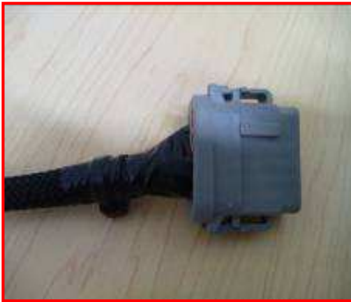
Figure 35: Wires taped on TMC Connector
