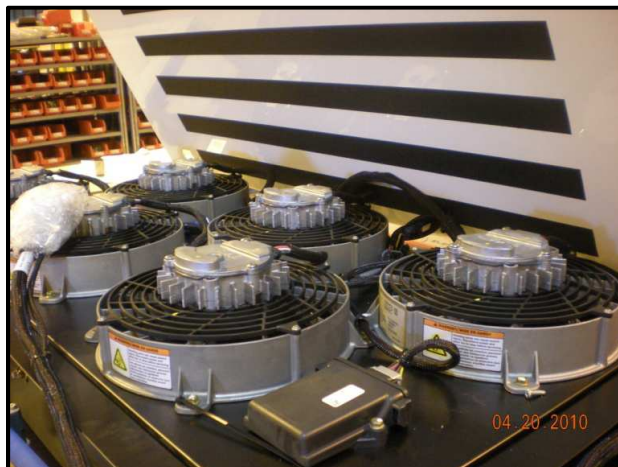
Figure 1: Rooftop Oil Cooler
