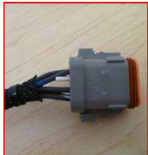
Figure 35: Wires exposed on J1939 Connector
