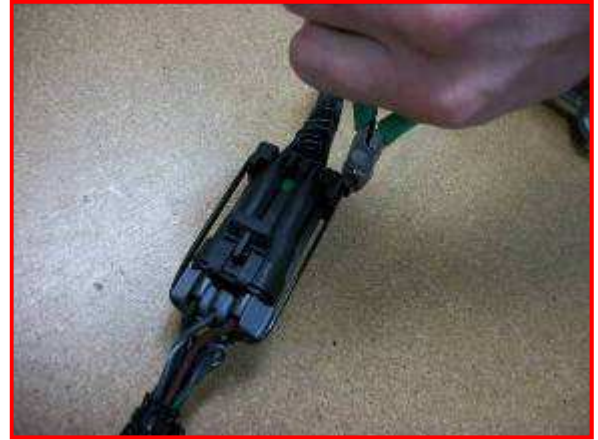
Figure 26: Zip Tie Secured and Trim
