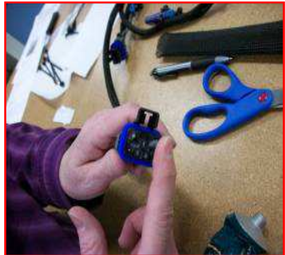
Figure 20: Smear Grease Over all Pins
