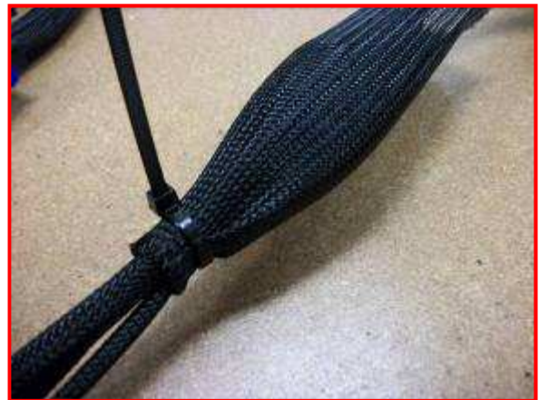
Figure 28: Zip Tie Protective Sleeve on Harness
