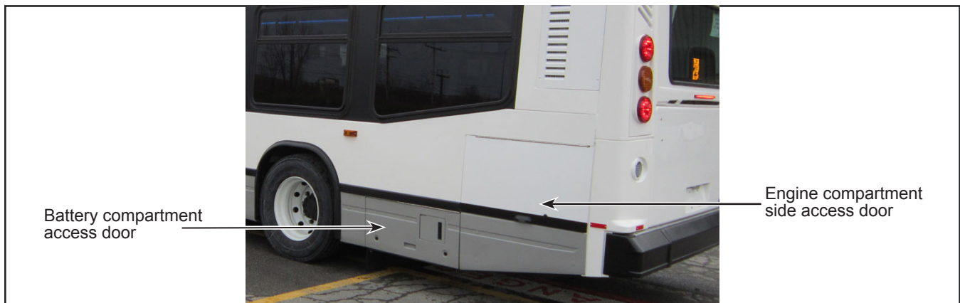
Figure 1 - Access Doors to Open
