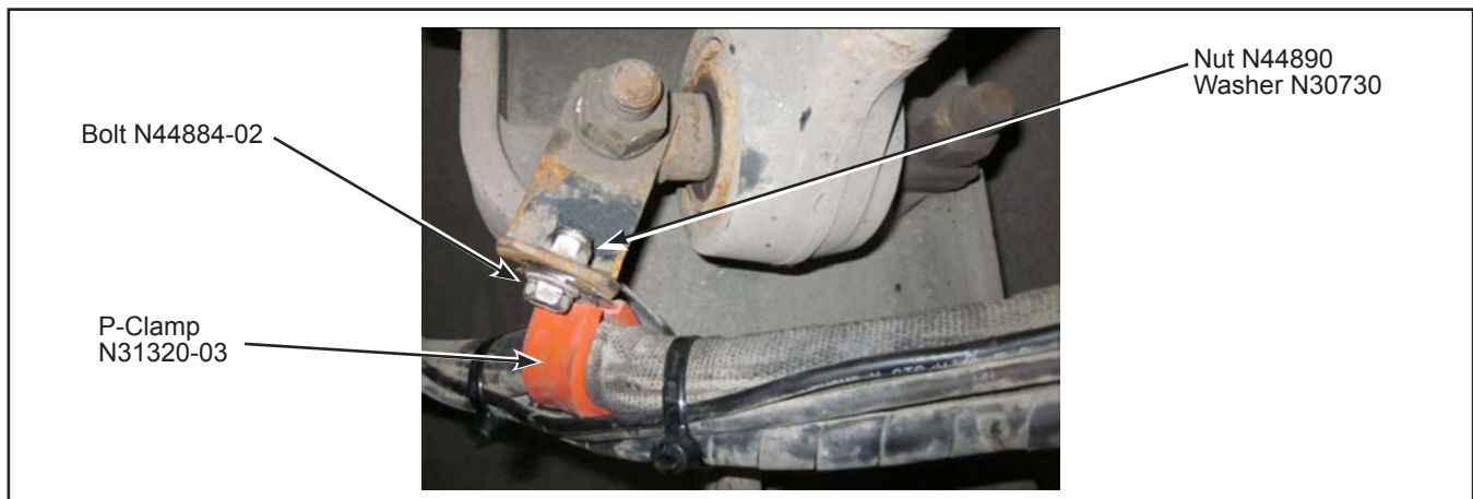
Figure 8 - L Support and P-Clamp Installation
