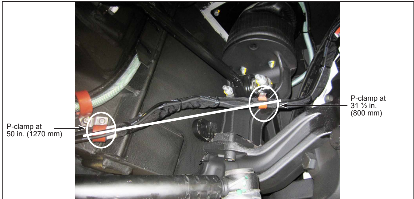
Figure 9 - P-Clamp Alignment at the 31½ in. (800 mm) and 50 in.(1270 mm) Positions
