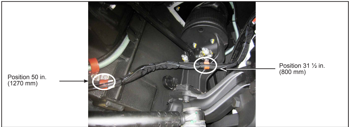
Figure 4 - P-Clamp Location on Hose
